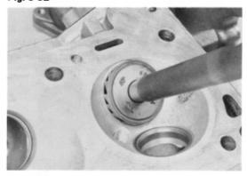
Resurface valve seats with 45° carbide cutter.
