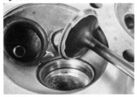
Coat valve face with prussion blue or white lead. Locate contact point on valve by rotating valve against seat.
